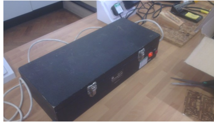
PCB exposed to UV light, transferring design
