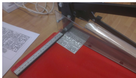
PCB cut to size using guillotine
