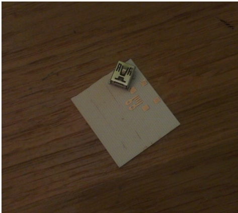
PCB and SMD Mini USB socket ready to be reflowed
