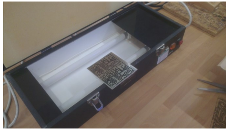
Design taped to photosensitive side of PCB
