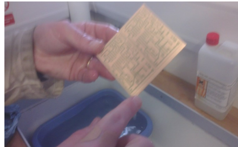
Design covers over copper in photoresist
