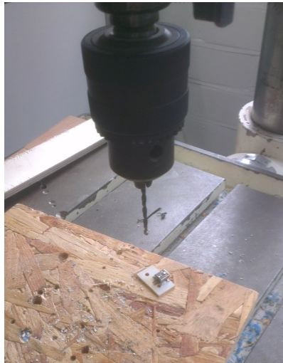
Drilling holes for PCB self adhesive stand offs
