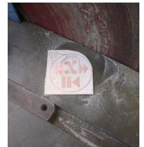
Board sanded using disc sander for rounded edges
