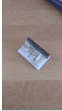
iPod connector breakout population
