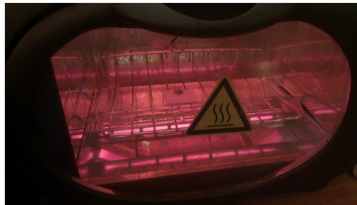
PCB being reflowed in a toaster oven
