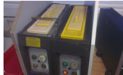
PCB put in bubble etch tank to remove unwanted copper
