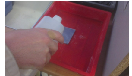
PCB developed removing unwanted photoresist
