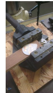
Larger holes for mounting drilled
