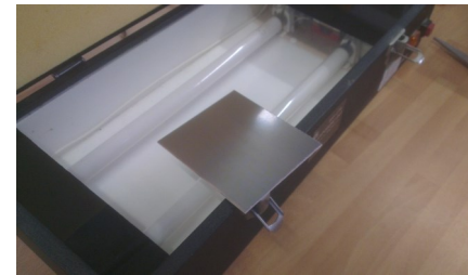
Design transferred to photoresist
