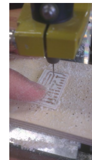
Holes drilled using 1mm drill bit
